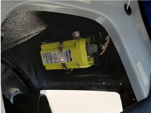
ELT transmitter location
