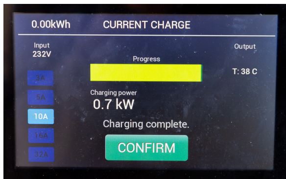
Charger display at the end of charging process
