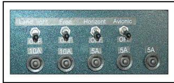
Example of switch and fuse layout
